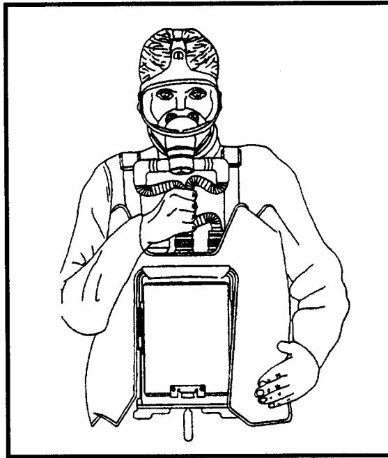
Figure 31-17. Testing OBA for leaks
